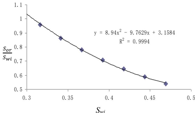
**Figure 1—Irreducible water saturation versus residual oil saturation relation.**
