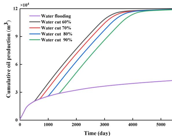
**Figure 14—Effect of different injection timing of compound flooding on cumulative oil production.**
