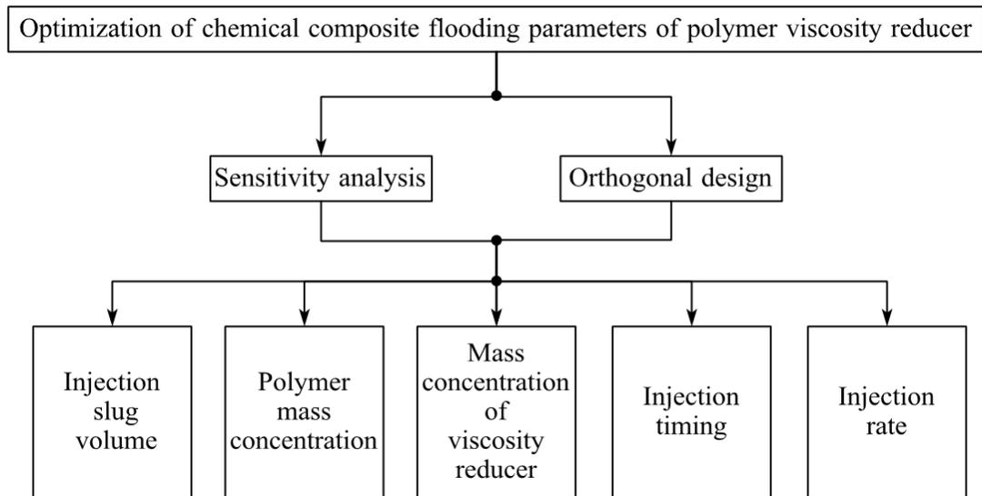
Figure 5—Simulation workflow.
