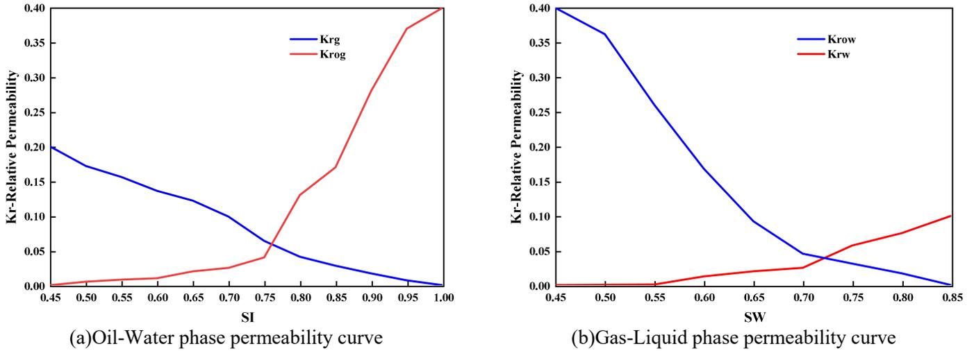
**Figure 2—Block relative permeability curves.**
