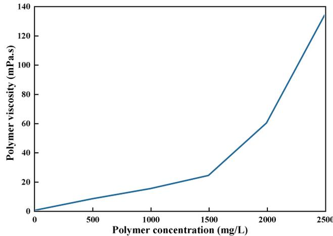
**Figure 3—Polymer viscosity-concentration curve.**
