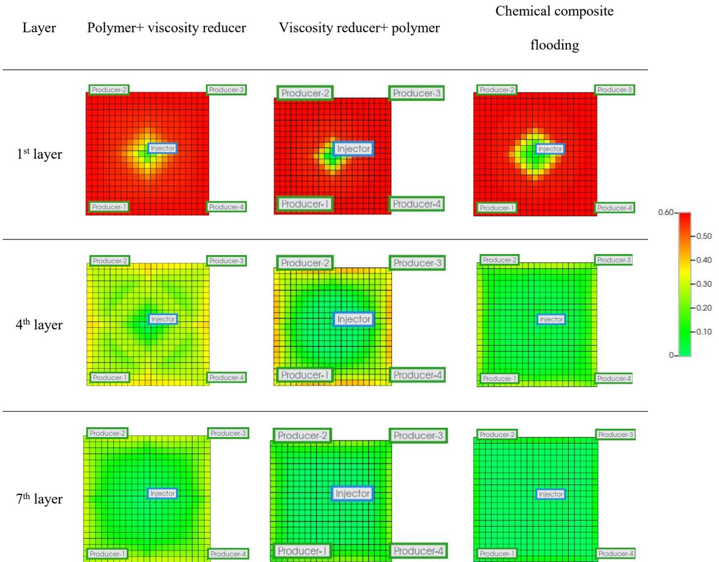
Figure 8—Oil saturation distribution for different injection methods.
