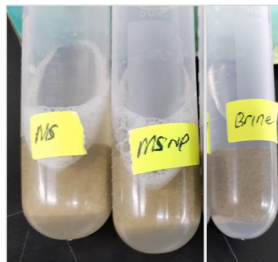
(b) Saturation of rock slice in MS, MS/SNPs and Brine solution
