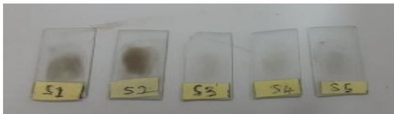
**Figure 4—Thin section of cores on glass slides.**
