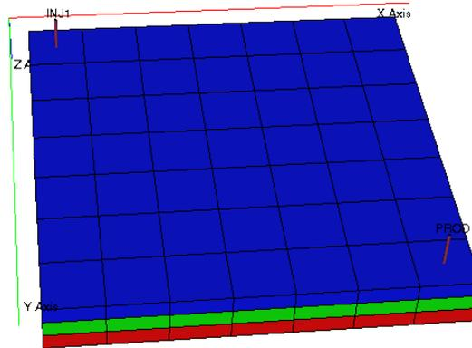
Figure 4—A three-dimensional reservoir model featuring INJ1 and PROD.
