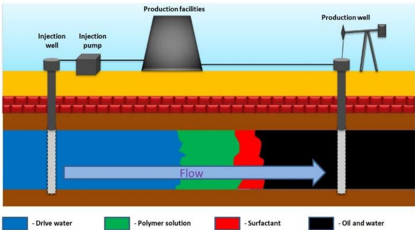
**Figure 2—Schematic of polymer flooding (Ragab and Mansour 2021).**
