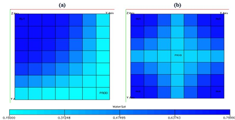
(a) direct line drive      (b) Five-spot pattern after polymer flooding
