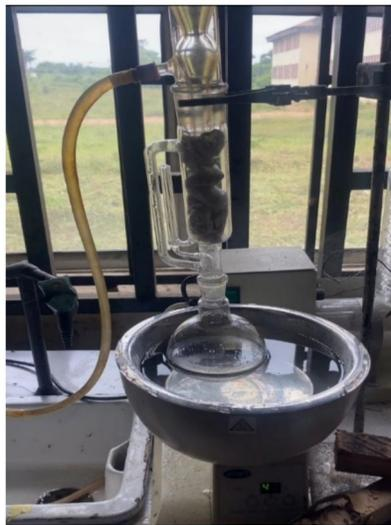
**Figure 3—Soxhlet extraction apparatus.**
