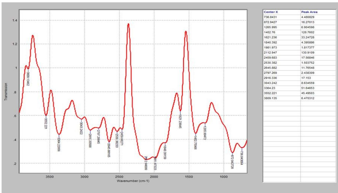
Figure 9—FTIR spectra for Sample B (Moringa Oleifera Seed).
