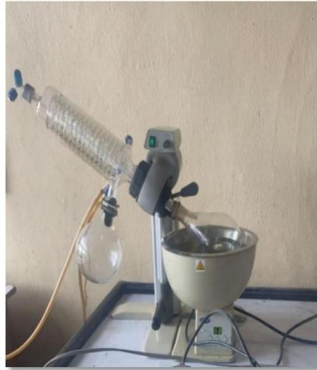
**Figure 4—Rotary evaporator.**
